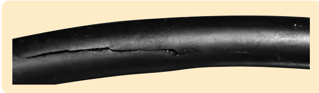
Figure 10-4: O-Ring Damaged by Explosive Decompression
