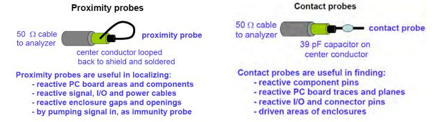
The proximity probe is moved around the enclosure or circuit board until an emission is located at the same frequency as the one found using the antenna. By locating the highest emission with the proximity probe, you have likely – but not definitely – located the source of the emission. The contact probe allows you to touch individual PC traces or component leads in searching for the frequency of interest.
